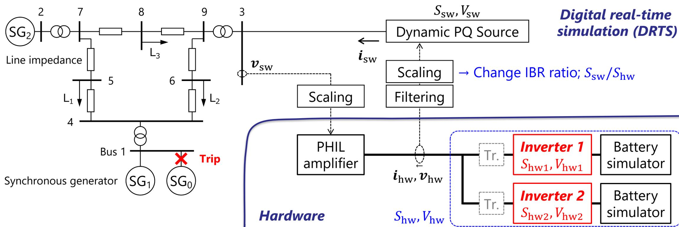
**How do we test multiple inverters with different ratings?**
