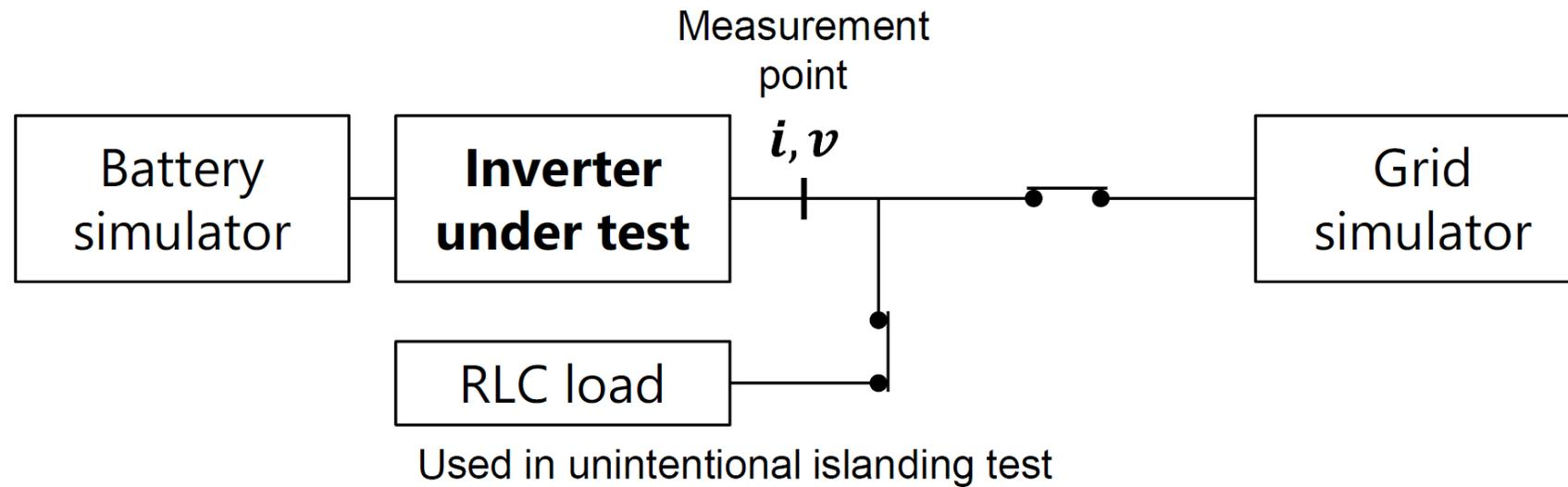
Fig. 5. Schematic diagram of the device connection configuration.
