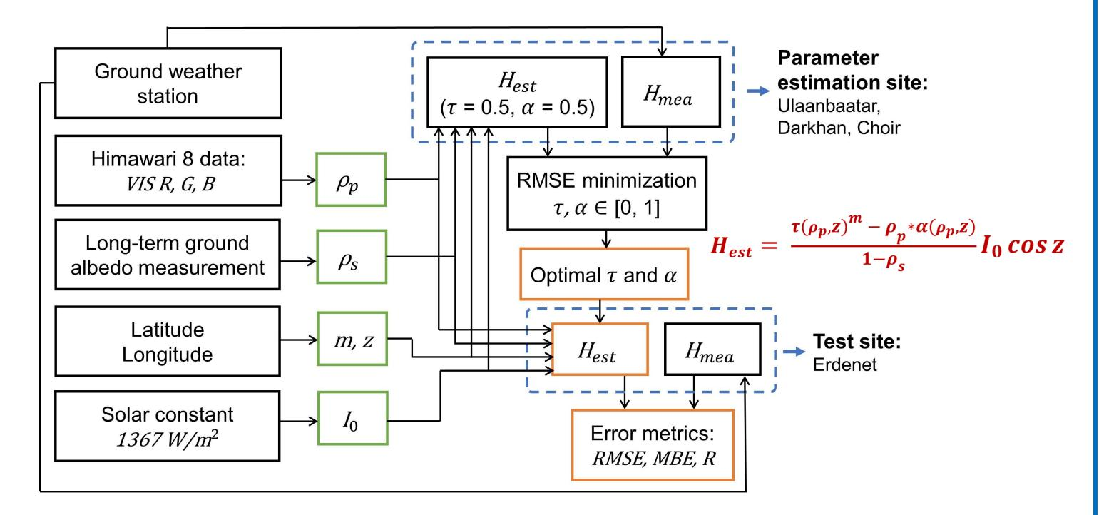
Schematics of the study design: inputs and outputs are shown in green and orange boxes, respectively. The equation to estimate the GHI is written in red.
